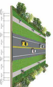
Typical Section #2 2-Lane Road with Sidewalks (Without Curb and Gutter)
