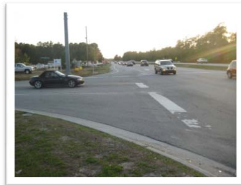
Consider offset stop bars at the westbound signal approach. Right turning vehicles would have better sight distance and southbound left-turning vehicles can turn more directly and efficiently.
