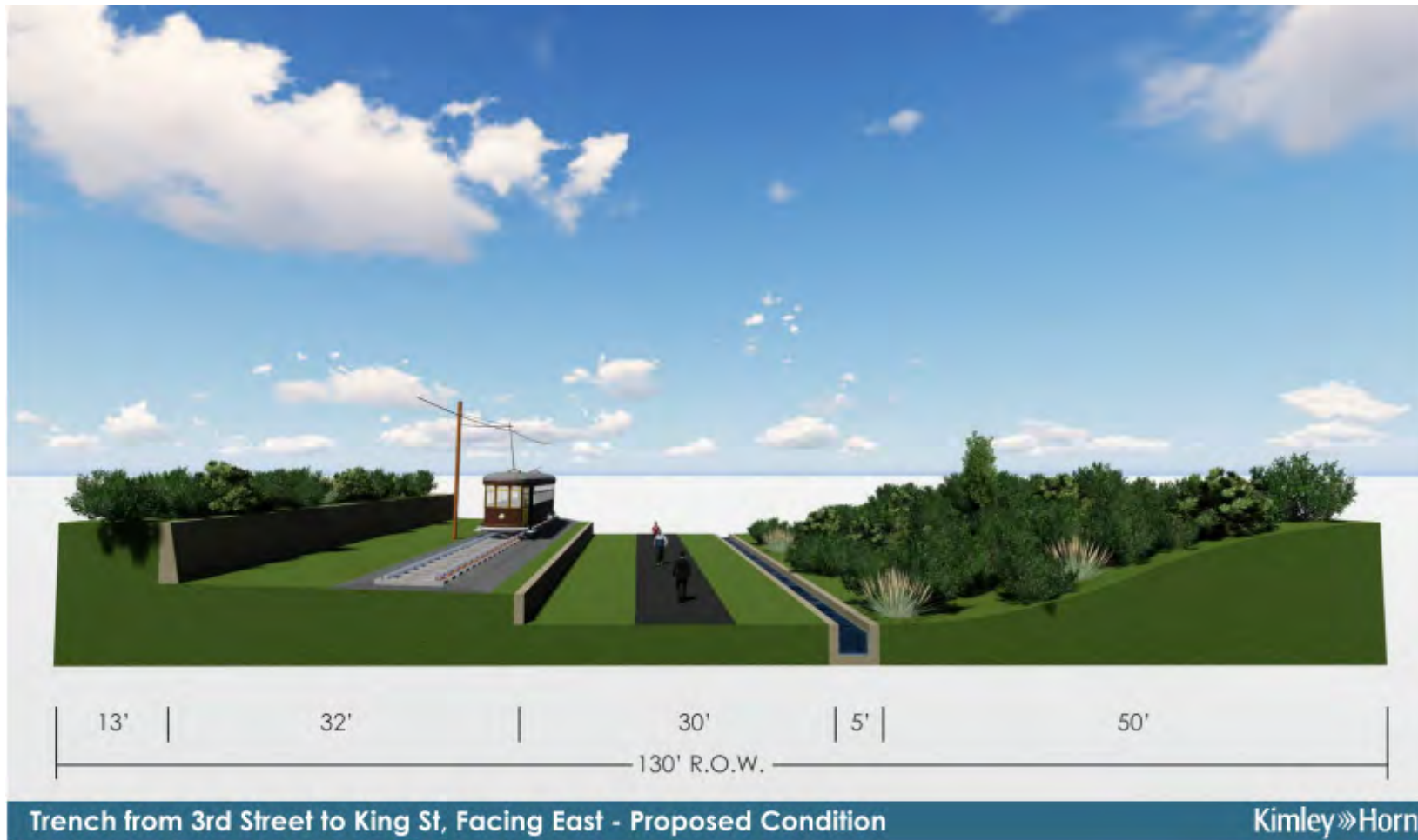
Figure A.1.2: PROPOSED CONDITION FOR TRENCH FROM 3RD STREET TO KING STREET SECTION
