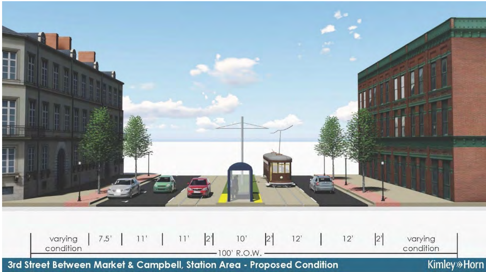
Figure A.7: PROPOSED IN-STREET STATION LAYOUT
