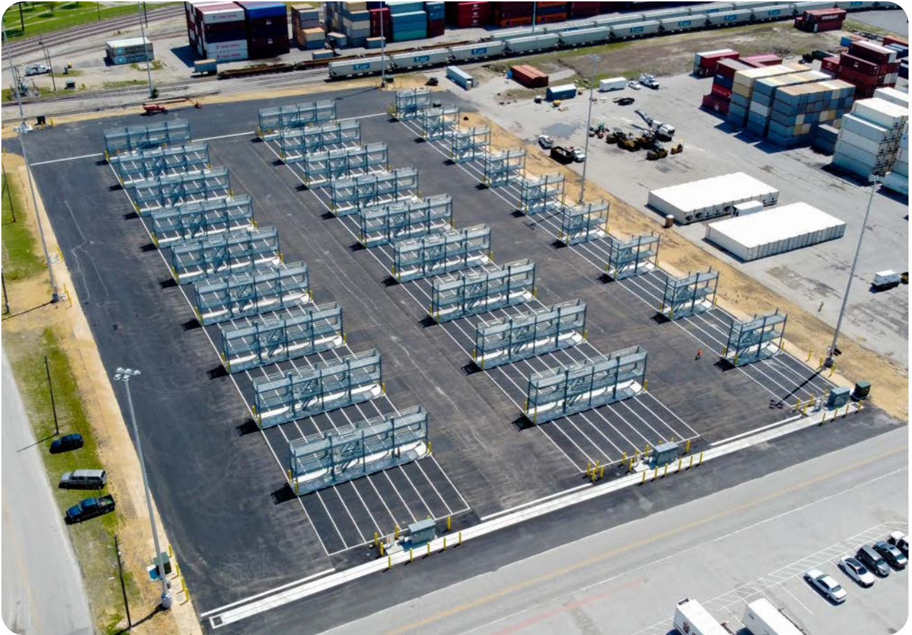
Above: The Port of Wilmington's new refrigerated container yard, completed in April 2020, has increased the Port's refrigerated container ("reefer") plugs from 235 to 775. Phase 2 of the project would allow the Port to expand to over 1,000 plugs. Photo Credit: North Carolina State Ports Authority
