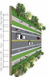
Typical Section #6 2-Lane Road with Sidewalks and Bike Lanes (With Curb and Gutter)
